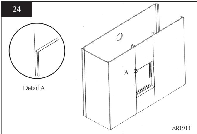
The top of the chimney breast must have a minimum 200cm<sup>2</sup> vent.
