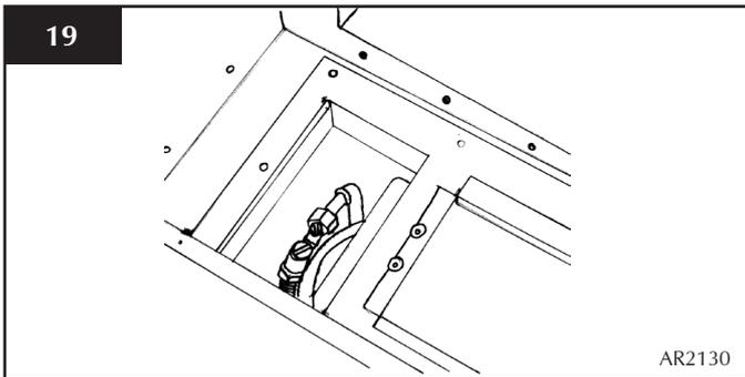
16.2 To leak test any gas joints on the appliance, the control assembly must first be undone and tilted backwards, see *Section 7, 7.3 Diagram 11*
