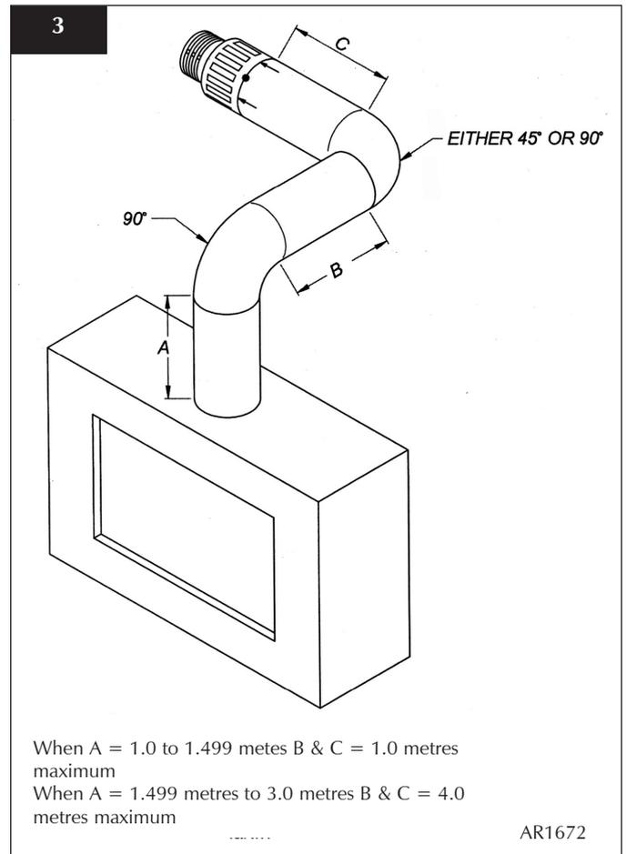
Any additional bend may be used on the horizontal section (either 45° or 90°), but the overall horizontal flue run will be reduced. Refer to Diagram 3.
