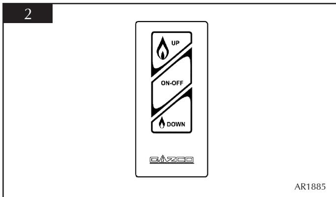
Press the ON-OFF button to light the appliance (up to 30 seconds). The UP button to increase the flame height.
