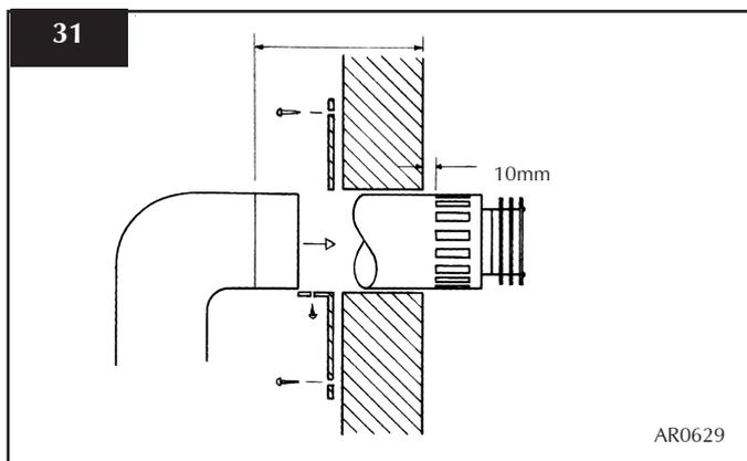
A wall plate is supplied to fix the flue to the wall:
