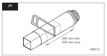
• Fit the flue to the appliance and secure with the aluminium tape supplied
