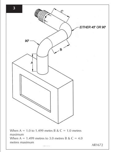
Any additional bend may be used on the horizontal section (either  $45^{\circ}$  or  $90^{\circ}$ ), but the overall horizontal flue run will be reduced. Refer to Diagram 3.
