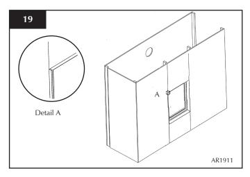
•Apply a plaster finish to the chimney breast
