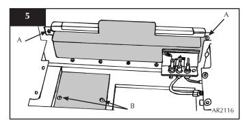
• Remove the two screws holding the access panel in place, Diagram 5, arrow B
