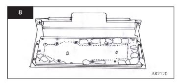
5.2 Place Log A onto the two studs on the burner skin, Diagram 9, with charred effect of the log facing forward.
