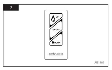
Press the ON-OFF button to light the appliance (up to 30 seconds). The UP button to increase the flame height.
