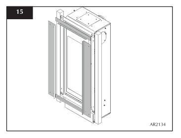
• Put vertical studwork at minimum clearance to the side of the fire (50mm)
