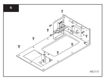
2.7 • Undo the 13 screws fixing the control unit in place
