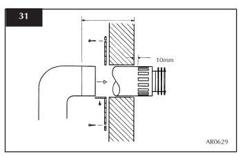
A wall plate is supplied to fix the flue to the wall:
