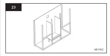
• Secure the top bracket at each side into the studwork using the screws provided
