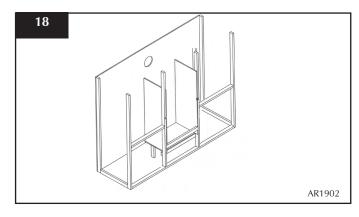
• Fit non-combustible board to the studwork above and to the sides of the fire. This should extend a minimum of 400mm above the appliance and a minimum of 50 mm to each side
