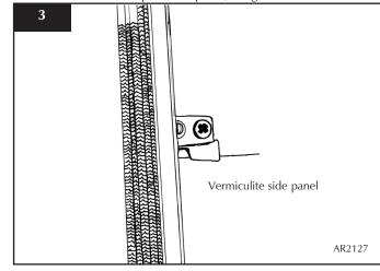
• Remove the two side panels and back panel and put to one side
