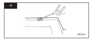
• Lift the glass clear from the lock bracket at the top of the frame and slide out
