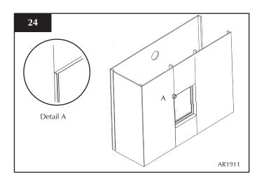
The top of the chimney breast must have a minimum  $200 \text{cm}^2$  vent.
