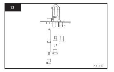
• Replace with a new electrode. Do not over-tighten the nut; this could break the component
