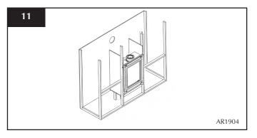
• Attach the 4 frame fixing brackets to the fire by placing the top part of the bracket through the slots
