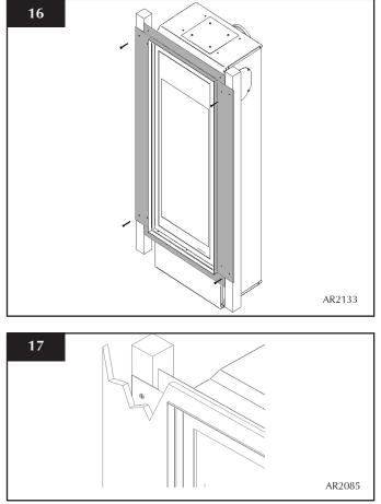
Build the studwork chimney breast to the desired size:
