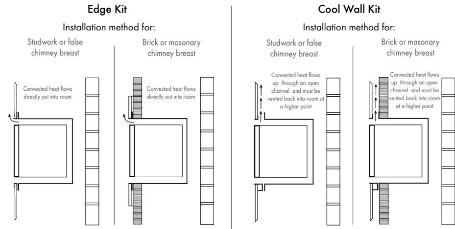
NB: When using the Edge Kit, heat resistant board and high temperature finishing plaster must be used. Please refer to installation instructions for full details of both kits which can be downloaded from [www.stovax.com](http://www.stovax.com)
