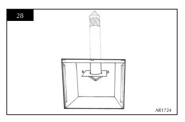
k) Inspect the debris deflector for damage and replace if necessary. Check the seal is intact, see *Servicing Requirements, Section 1* and replace if necessary.
