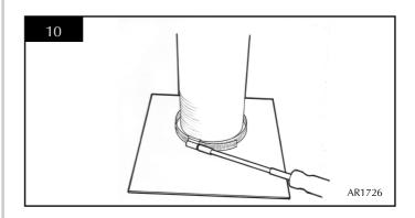
5.9.3 Secure the flue spigot plate to the inside top surface using the eight screws provided. Diagram 9.
