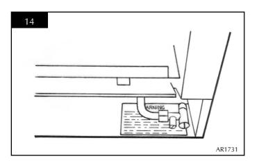
5.14 Locate the top of the inner box into the runners at the top of the outer box. Diagram 15.
