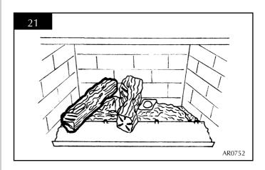
7.5 Place log 4 on the right-hand side of the centre log. There is a large recess on the underside of the log, which is located on log 1. See diagram 22.
