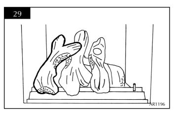
7.13 Place log E on the last stud. The recess on the underside of the log should locate on to the top of log D. See diagram 30.
