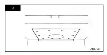
5.9.2 Pull the liner through the hole in the top of the outer box and attach it to the flue spigot plate using the clip provided. Tighten the clip securely. Diagram 10.
