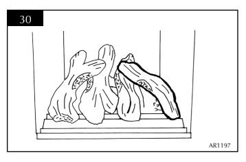
7.14 Place log F on the rear tray and leaning forward to locate in the recess in log E. See diagram 31.
