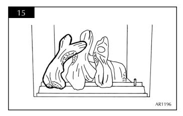
6.13 Place log E on the last stud. The recess on the underside of the log should locate on to the top of log D. See diagram 16.
