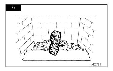
6.4 Place log 3 on the far left-hand stud. The recess on the underside of the log should locate on the top of log 1 on the far left-hand side. See diagram 7.
