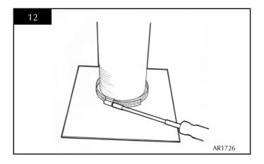
5.12 Push the Debris Deflector up into the chimney and secure the flue spigot plate to the inside top surface using the eight screws provided. Diagram 13.
