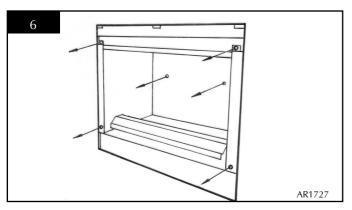
5.6 Slide the inner box away from the outer box by pulling it forward. Diagram 7
