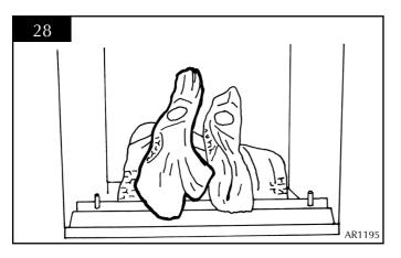
7.12 Place log B on the first stud. The recess on the underside of the log should locate on the top of log C. See diagram 29.
