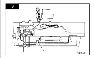
8.3 Reassemble the thermocouple into the rear of the valve. DO NOT OVERTIGHTEN. Check for leaks after reassembly.
