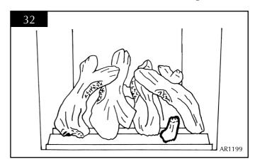
7.16 With the granules fill the front compartment around the logs evenly. ENSURE NO GRANULES FALL ON THE BURNER. See diagram 33.
