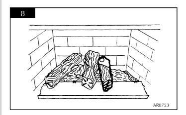
6.6 Place log 5 on top of log 4 and ensure the two large locations engage. Locate the front of the log on to the far right-hand stud. See diagram 9.
