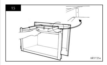
5.15 Gently slide the inner box into the outer box until the two flanges meet. Secure with the screws on the flange and the two screws on the inside rear surface as shown.
