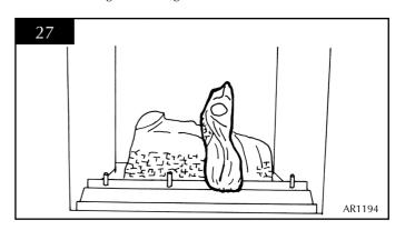
7.11 Place log C on the second stud resting at the rear on log A. See diagram 28.
