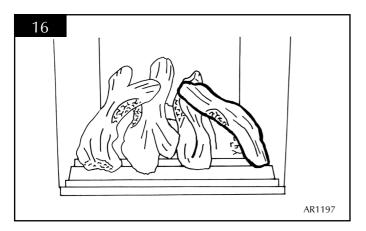
6.14 Place log F on the rear tray and leaning forward to locate in the recess in log E. See diagram 17.
