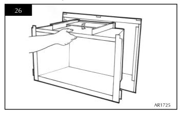
j) Undo the eight screws securing the flue spigot plate to the inside top surface. See Diagram 27.
