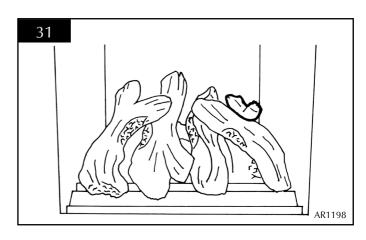
7.15 Place log G at the front of the fire between logs D and E. DO NOT PLACE THIS LOG ON THE BURNER. IT IS ONLY TO FILL THE GAP BETWEEN LOGS D AND E. The charred effect should face the rear of the fire. See diagram 32.
