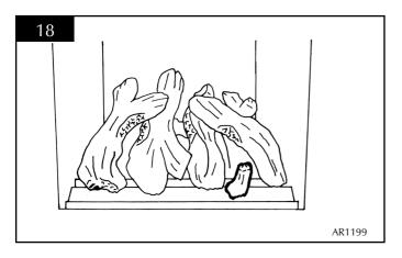
6.16 With the granules fill the front compartment around the logs evenly. ENSURE NO GRANULES FALL ON THE BURNER. See diagram 19.
