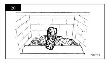
7.4 Place log 3 on the far left-hand stud. The recess on the underside of the log should locate on the top of log 1 on the far left-hand side. See diagram 21.
