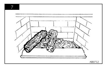
6.5 Place log 4 on the right-hand side of the centre log. There is a large recess on the underside of the log, which is located on log 1. See diagram 8.
