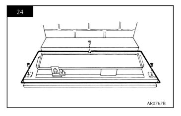
h) Remove the four screws securing the inner to the outer box and undo the two screws behind the rear ceramic panel. Diagram 25.
