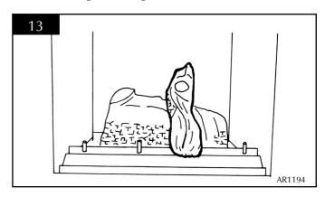
6.11 Place log C on the second stud resting at the rear on log A. See diagram 14.
