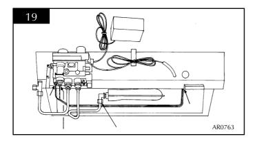
9.2 Rotate the injector until it is fully removed, and install the correct replacement injector. Re-assemble and turn the gas supply on, check for any leaks.
