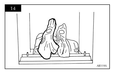
6.12 Place log B on the first stud. The recess on the underside of the log should locate on the top of log C. See diagram 15
