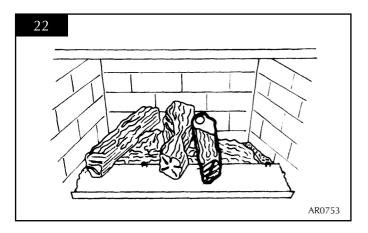
7.6 Place log 5 on top of log 4 and ensure the two large locations engage. Locate the front of the log on to the far right-hand stud. See diagram 23.
