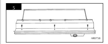
i) Remove the two screws at the front of the burner tray and loosen the screw at the rear. See diagram 6.
