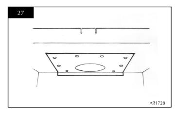
k) Pull the debris deflector down and out of the chimney and inspect the space immediately above the appliance for a build up of debris. See Diagram 28.
