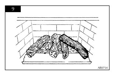
6.7 Place log 6 on the remaining stud and lean the log on to log 1 between logs 2 and 3. There is a notch to locate the log. See diagram 10.
