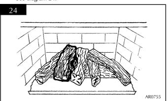
7.8 Place log 7 at the front of the fire between logs 4 and 5. DO NOT PLACE THIS LOG ON THE BURNER. IT IS ONLY TO FILL THE GAP BETWEEN LOGS 4 AND 5. The charred effect should face the rear of the fire.
