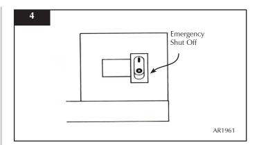
(This switch is set to be ON (|) during normal operation and must remain ON)
