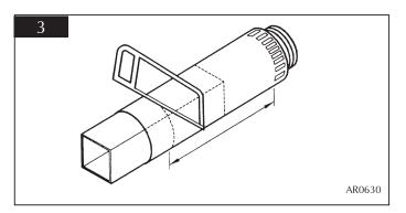
2.8 Attach the flue to the appliance and seal using the aluminium tape. See diagram 4.
