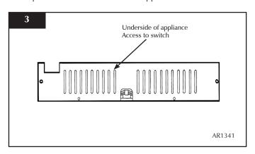
• Use a ball point pen or narrow screwdriver to push the rocker switch to the OFF (O) position, Diagram 4
