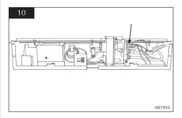
9.4 Support the valve and remove the magnetic valve retaining nut, Diagram 11
