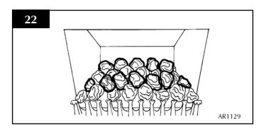
6.13 Place the remaining 5 small coals on top of the others so that they form a bridge between the second and third rows. See Diagram 23.
