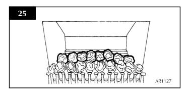
6.16 Place 7 large coals so that they form a bridge between the other 2 rows, and 2 small coals, 1 at each end. Place 6 large coals at the back of the fire. See Diagram 26.
