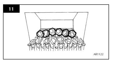
7.12 Place 5 large coals so that they form a bridge between the other 2 rows, then 2 small coals, 1 at each end. Place 5 large coals at the back of the fire. See Diagram 12.
