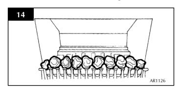
7.15 Place 8 large coals onto the flame baffle fingers. See Diagram 15.
