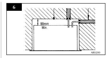
Note: Gas pipes passing through masonry must be protected.
