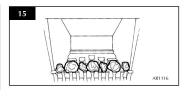
6.6 Place 5 large coals onto the flame baffle fingers. See Diagram 16.
