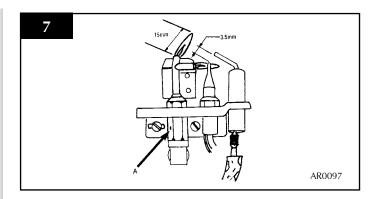
5.6 After reassembly, check for gas soundness and carry out a flame failure functional check details in the flow chart, especially the mag drop out time.
