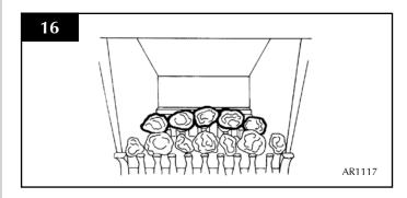
6.7 Place 4 large coals so that they form a bridge between the other 2 rows, and 2 small coals, 1 at each end. Place 4 large coals at the back of the fire. See Diagram 17.
