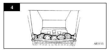
7.5 <u>Flat fronts (All others)</u> - Place 3 large coals and 4 small coals onto the front coal moulding ensuring that they rest against the decorative front, these should run intermittently small, large, small etc. See Diagram 5.
