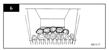
7.7 Place 4 large coals so that they form a bridge between the other 2 rows, and 2 small coals, 1 at each end. Place 4 large coals at the back of the fire. See Diagram 7.
