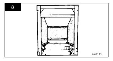
5.5 Fit the gas pipe into position, ready for passing into the convector box, ensuring enough remains to connect to the fire.
