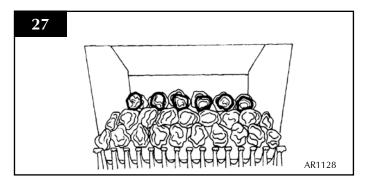
6.17 Place the remaining 6 small coals on top of the others so that they form a bridge between the second and third rows. See Diagram 27.
