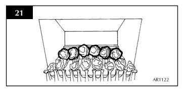
6.12 Place 5 large coals so that they form a bridge between the other 2 rows, and 2 small coals, 1 at each end. Place 5 large coals at the back of the fire. See Diagram 22.
