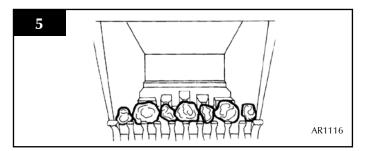
7.6 Place 5 large coals onto the flame baffle fingers. See Diagram 6.
