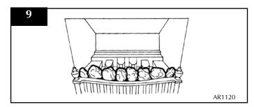
7.10 Flat fronts (All others) - Place 4 large coals and 4 small coals onto the front coal moulding ensuring that they rest against the decorative front, these should run intermittently small, large, small, with 2 large in the centre. See Diagram 10.
