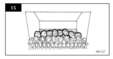
7.16 Place 7 large coals so that they form a bridge between the other 2 rows, and 2 small coals, 1 at each end. Place 6 large coals at the back of the fire. See Diagram 16.
