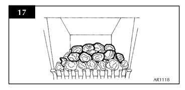
6.8 Place the remaining 4 small coals on top of the others so that they form a bridge between the second and third rows. See Diagram 18.
