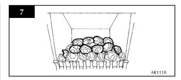
7.8 Place the remaining 4 small coals on top of the others so that they form a bridge between the second and third rows. See Diagram 8.
