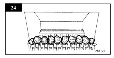
6.15 Place 8 large coals onto the flame baffle fingers. See Diagram 25.
