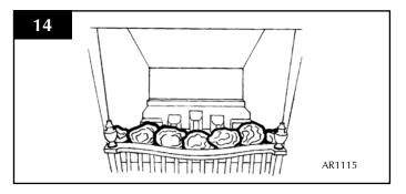
6.5 Flat fronts (All others) - Place 3 large coals and 4 small coals onto the front coal moulding ensuring that they rest against the decorative front, these should run intermittently small, large, small etc. See Diagram 15.
