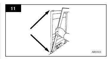
5.13 Fit the fret to the fire front using the two securing screws. See Diagram 12.
