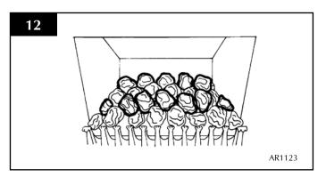
7.13 Place the remaining 5 small coals on top of the others so that they form a bridge between the second and third rows. See Diagram 13.
