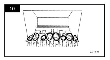
7.11 Place 6 large coals onto the flame baffle fingers. See Diagram 11.
