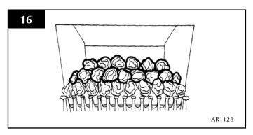
7.17 Place the remaining 6 small coals on top of the others so that they form a bridge between the second and third rows. See Diagram 17.
