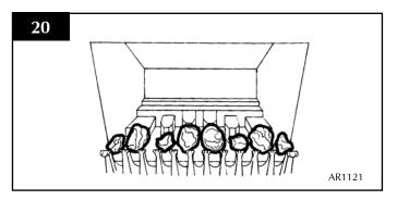
6.11 Place 6 large coals onto the flame baffle fingers. See Diagram 21.
