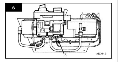
5.5 Replace with a new pilot assembly. Set the spark gap. See Diagram 7.
