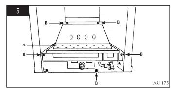
6.2 Position the flame baffle centrally on the tray and ensure the stepped lower edge engages against the rear edge of the burner skin. See diagram 6.
