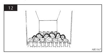
6.9 Place one small coal either side on top of the flame baffle in each rear corner. Then place two large coals in between the two small coals. These coals should touch the rear panel. See diagram 13.
