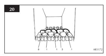
7.15 Place the rear row of pebbles on top of the flame baffle, these must touch the rear panel. See diagram 21.
