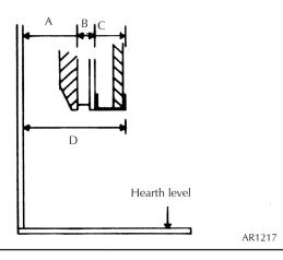
When fitting the Logic Convector fire and a Stovax Cast Iron Convector fireplace to a precast letter box flue with a standard starter block, the 8315 spacer kit will be required, together with an extra deep 142mm rebate surround.
