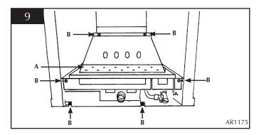
7.2 Position the flame baffle centrally on the tray and ensure the stepped lower edge engages against the rear edge of the burner skin. See diagram 10.
