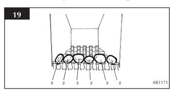
7.14 Working from the outer edges, place the second row of pebbles against the rear of the first row. Note the orientation of each pebble, as this is important to the performance of the fire. See diagram 20.
