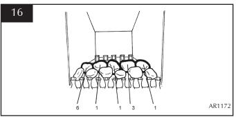
6.15 Place the rear row of pebbles on top of the flame baffle, these must touch the rear panel. See diagram 17.
