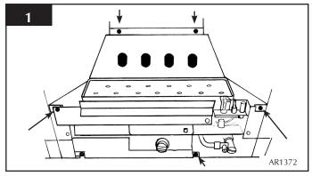
1.7 The burner unit can now be removed.
