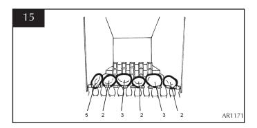
6.14 Working from the outer edges, place the second row of pebbles against the rear of the first row. Note the orientation of each pebble, as this is important to the performance of the fire. See diagram 16.
