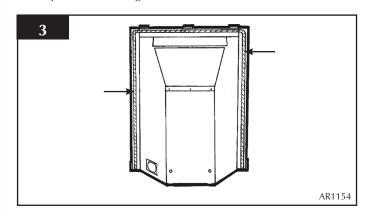
5.4 Gas pipe entry must come through the right hand side of the box. The rubber seal must be cut using a sharp knife to allow the isolating elbow to pass through it. Ensure the rubber is not damaged when doing this.
