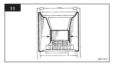
7.4 Locate the top panel on top of the rear and side panels. Finally push the sides fully towards the rear panel. This will retain the top panel. See diagram 12.
