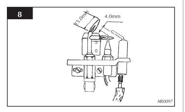
4.6 After reassembly, check for gas soundness and carry out a flame failure functional check details in the flow chart, especially the mag drop out time.
