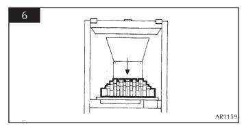
6.3 Place the rear panel against the rear of the box and slide the side panels on either side of the flame baffle. Ensure they locate in the brackets at the top of the firebox. DO NOT SLIDE THEM ALL THE WAY BACK. See diagram 7.
