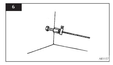
6.7 Coil up the surplus cable and locate in the back of the fire box.
