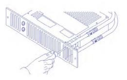
4. Isolate electrical supply and connect the transformer flying leads to the fused spur (3A). The transformer must be located outside the bathroom or high humidity area. Connect the single-pin male connectors to the twin core cable you have supplied.
