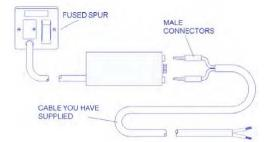
5. Push in the connectors to the transformer terminals and connect the other end of the cable to the terminals on the back of the product.
