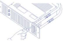
Isolate electrical supply and connect the heater electric cable to the fused spur (3A). Ensure the fused spur is not directly above the heater and is accessible after installation is complete.
