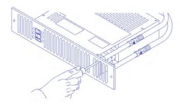
4. Isolate electrical supply and connect the heater electric cable to the fused spur (5A). Ensure the fused spur is not directly above the heater and is accessible after installation is complete.
