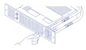
4. Isolate electrical supply and connect the heater electric cable to the fused spur (3A). Ensure the fused spur is not directly above the heater and is accessible after installation is complete.
