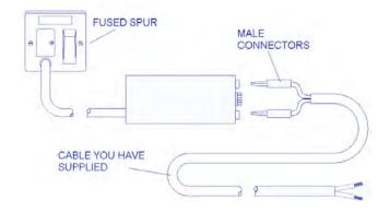
Push in the connectors to the transformer terminals and connect the other end of the cable to the terminals on the back of the product.
