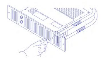
4. Isolate electrical supply and connect the transformer flying leads to the fused spur (3A). The transformer must be located outside the bathroom or high humidity area. Connect the single-pin male connectors to the twin core cable you have supplied.
