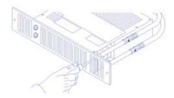
5. Isolate electrical supply and connect the transformer flying leads to the fused spur (3A). The transformer must be located outside the bathroom or high humidity area. Connect the single-pin male connectors to the twin core cable you have supplied.
