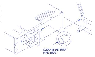
3. Connect the flexible hoses (the ends that include the isolating valves) to the heater flow and return pipes. Connect the other ends of the flexible hoses to the heating system flow and return pipes. If the connections are correct the marks you made on the pipes will **NOT** be visible. Open the valves and check for leaks. To remove the flexible hoses see page 23.
