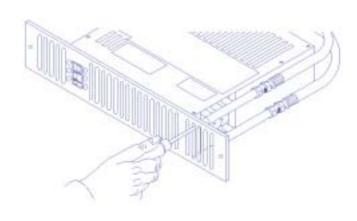
5. Isolate electrical supply and connect the heater electric cable to the fused spur (5A). Ensure the fused spur is not directly above the heater and is accessible after installation is complete.
