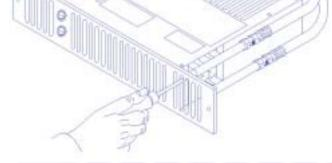
5. Isolate electrical supply and connect the heater electric cable to the fused spur (3A). Ensure the fused spur is not directly above the heater and is accessible after installation is complete.
