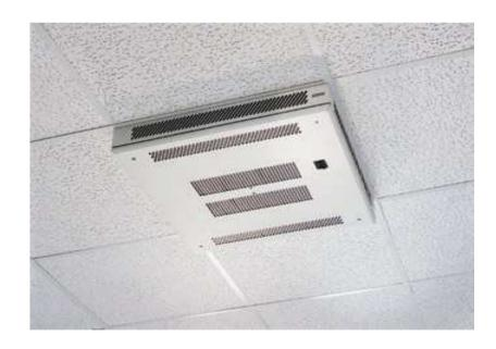
The heater appliance is designed to fit either directly to the ceiling or suspended through a 600mm x 600mm tile surround. The MAXIMUM recommended height from floor to underside of unit must not exceed 3.2 metres. When installing in a suspended ceiling the appliance must be supported by chains or threaded rods. Do not attempt to fix the unit to the ceiling tile frame.
