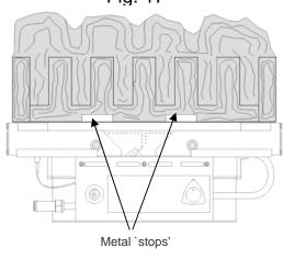
The support shelf is positioned on the fibre support metalwork. There are two metal `stops' that prevent the support shelf from sitting on the main burner outlet (Fig. 3).
