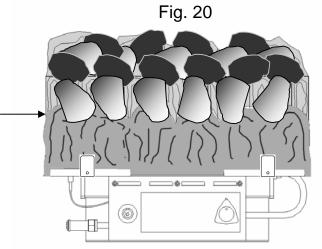
To obtain the best visual appearance, it may be necessary to `slightly' adjust the position of the coals. If any of the coals or coal bed become damaged or lost, replacements MUST be obtained before further use.
