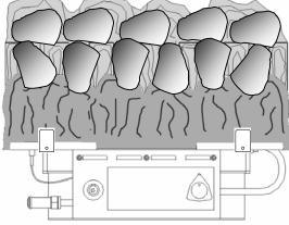
Place 6 large coals/pebbles on top of the simulated front (one in each groove). Allow the coals/pebbles to rest on the support shelf. Place 5 large coals/pebbles on the on the first tier of the support shelf (Fig. 5).
