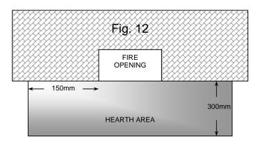
Minimum hearth height - 50mm Minimum hearth width - 805mm Minimum hearth thickness - 12.5mm
