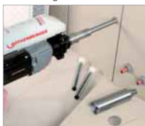
Clean drilling of tiles
