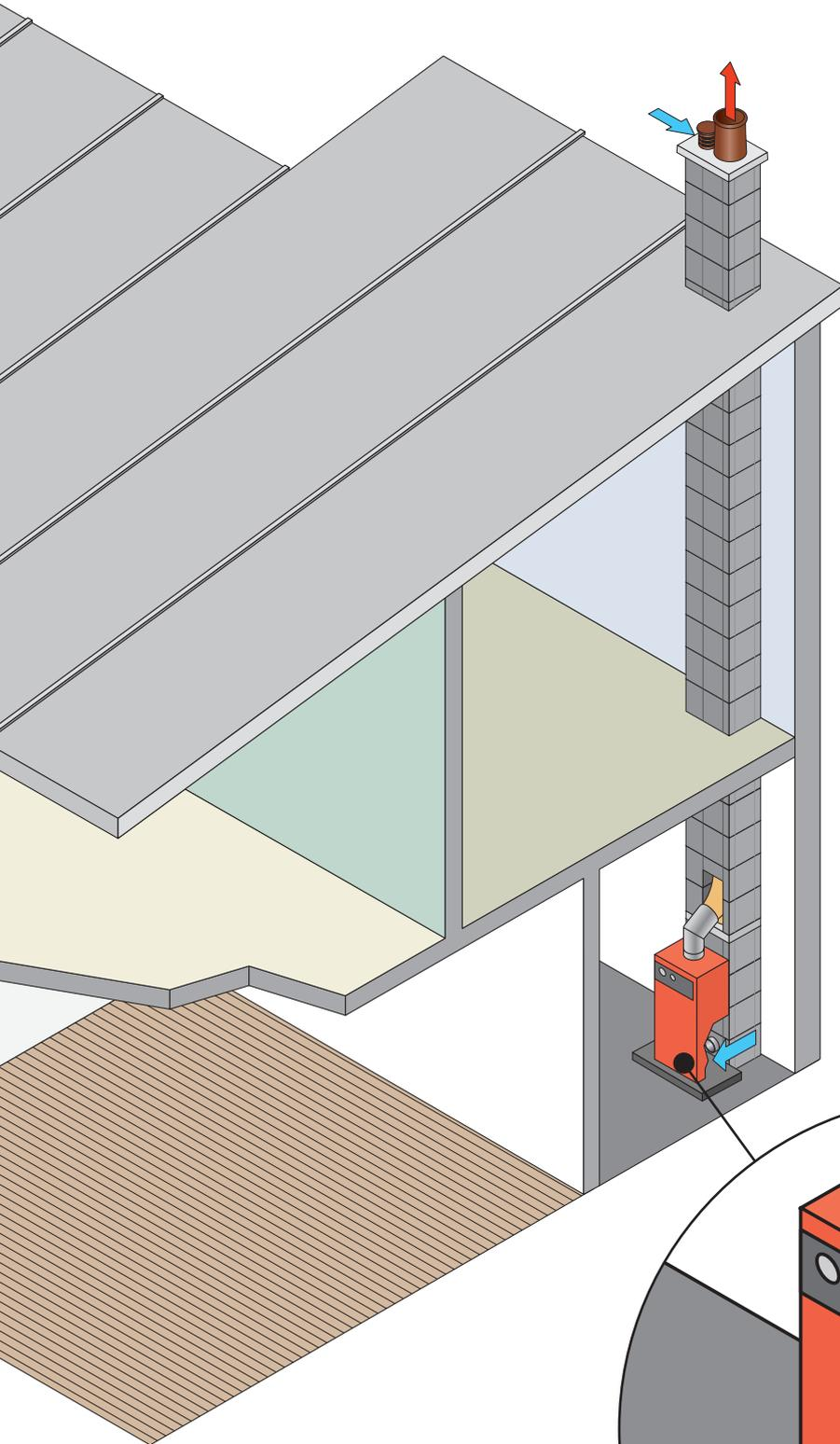
Combustion air is supplied directly to the boiler from outside the house.
