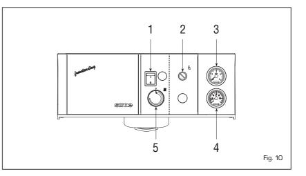
immediately turning off the burner when the boiler accidentally overheats. To restore normal operations, wait until the temperature drops below the thermostat calibration setting.
