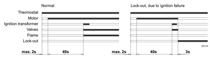
When flame-failure occurs during working, shut down takes place within one second.
