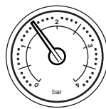
Fig. 11 Normal Pressure (operating)
