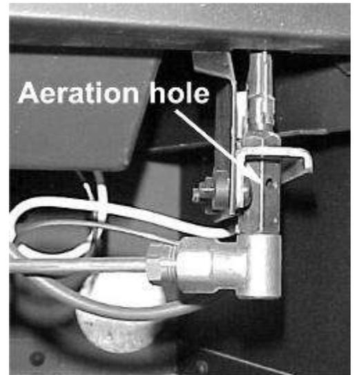
**Note: - Take care when cleaning in this area so as not to damage the pilot assembly.**
