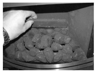
Now place the right side of the fuel bed in position behind the front ledge of the tray as shown above. Finally place the small back liner board in place behind the fuel bed to cover the metal bracket behind.
