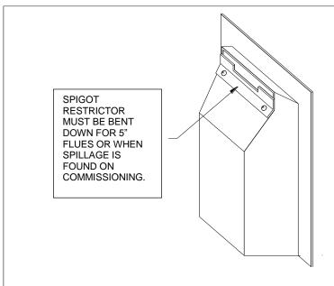
**Note:** A brick or stone chimney with a 125 mm (5 ins) minimum diameter flue liner conforming to BS 715 may be used. Provided a suitable sealing plate is fitted to the base of the liner and the appliance does not restrict the opening into the liner.
