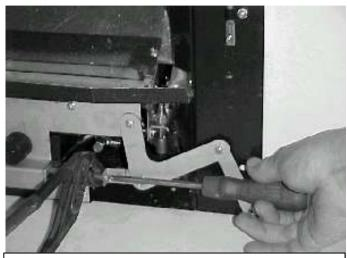
Taking great care grip the copper protective sleeve at the end of the gas control spindle (DO NOT GRIP SPINDLE IN ANY OTHER PLACE) as shown and remove the screw from the end as shown above.
