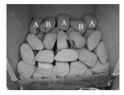
\* Before fitting the pebble set loosen the burner securing screws and make sure that burner is pushed to the right side of the burner tray. This will ensure maximum aeration to the burner and reduce discolouration.
