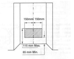
Drill holes for eye bolts on 112mm centre lines between maximum and minimum heights.
