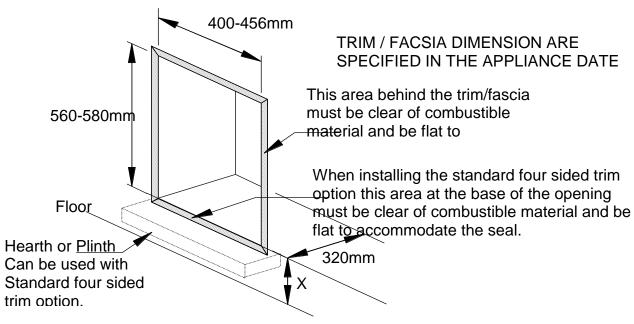
The front face and the base of the fire opening must be flat to ensure that a good seal is formed between the rear and base of the appliance and the chimney to avoid any reduction of natural draught.
