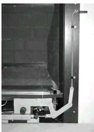
Connect the link lever to the stud at the end of the slide control lever and replace the nylock nut. IMPORTANT TURN THE NUT UNTIL IT JUST TIGHTENS AND THEN TURN IT BACK A HALF TURN. Check the operation on the lever and mechanism ensure that the lever springs back to the low position when it is released after pushing down.
