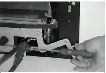
Taking great care grip the copper protective sleeve at the end of the gas control spindle (DO NOT GRIP SPINDLE IN ANY OTHER PLACE) as shown and remove the screw from the end as shown above.
