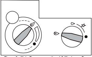
Figure 9 - Main Burner operational & Maximum Gas Rate
