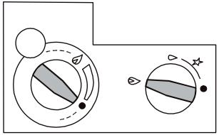
Figure 8 - Main burner operational, but gas flow off
