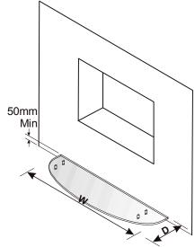
Figure 56 – Example of physical barrier (dimensions as stated in Table 3 – Protected Area)
