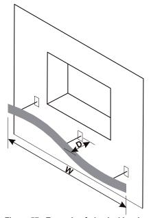
Figure 57– Example of physical barrier (dimensions as stated in Table 3 – Protected Area)
