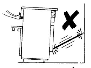
Release the stability chain as you ease the cooker out. Don't forget to refit it when you replace the cooker.
