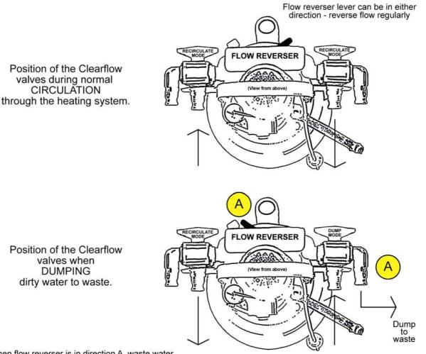
When flow reverser is in direction A, waste water will be expelled through dump valve A.
