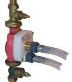
2c. Across the "tails" of a radiator (having drained and disconnected the radiator) using appropriate 1/2" or 3/4" BSP adaptors to connect to the valves. The radiator valves should be closed to isolate the flushing pump from the system until
