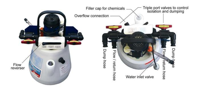
1b. The Clearflow CF30 Hyper-Jet has two 3 metre flow and return hoses, fitted with black re-inforced plastic 'cup type' quick release hose connections on one end, and <sup>3</sup>/<sub>4</sub>" female brass hose connectors on the other end of each hose.
