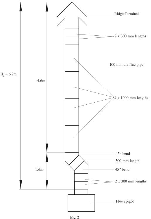
Worked example of equivalent flue height
