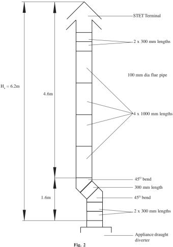
Worked example of equivalent flue height
