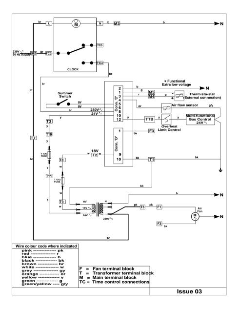
Fig. 6a, MODAIRFLOW FUNCTIONAL DIAGRAM
