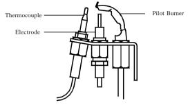
Fig. 3 Pilot Burner Assembly
