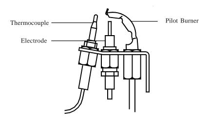
Fig. 3 PILOT BURNER ASSEMBLY
