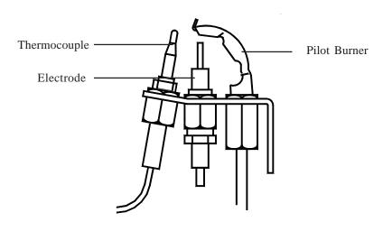
Fig. 3 PILOT BURNER ASSEMBLY
