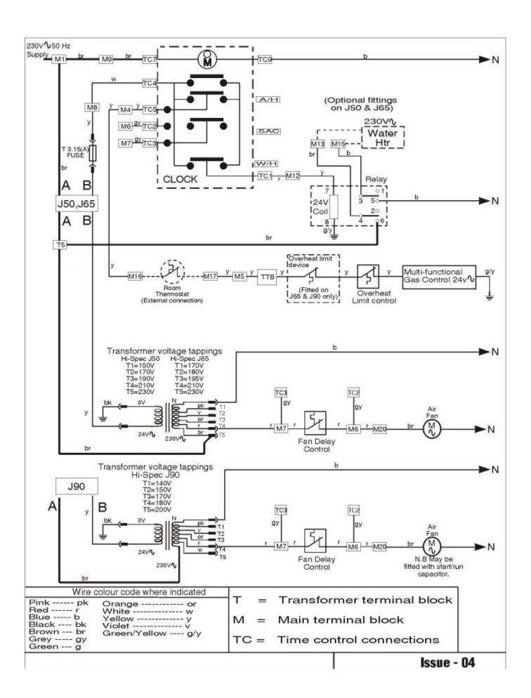
Fig. 6b, non-MODAIRFLOW FUNCTIONAL DIAGRAM
