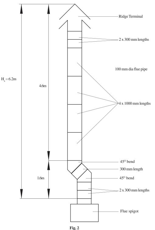
Worked example of equivalent flue height
