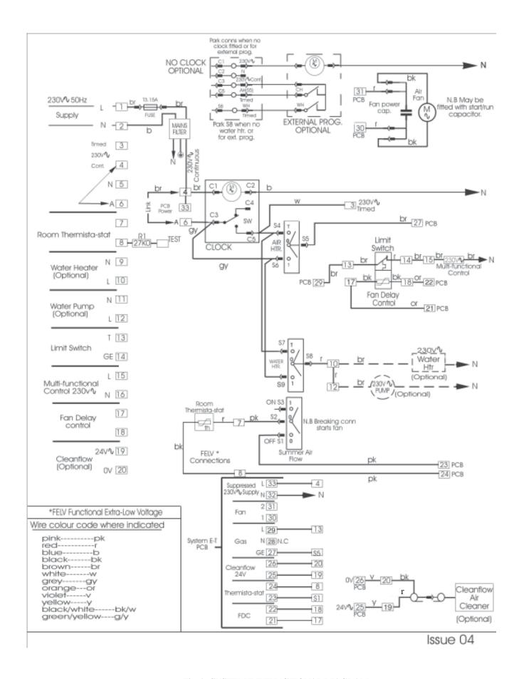
Fig. 6a, SYSTEME-TFUNCTIONAL DIAGRAM
