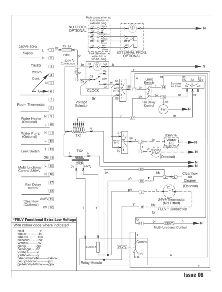
Fig. 6b, BASIC CONTROL FUNCTIONAL DIAGRAM
