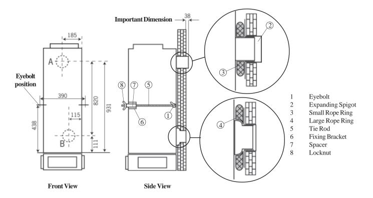
Fig. 2 HI-SPEC J25RS fitted to SE-Duct - fitting dimensions
