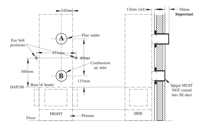
Fig. 2 HI-SPEC J25RS fitted to SE-Duct - fitting dimensions
