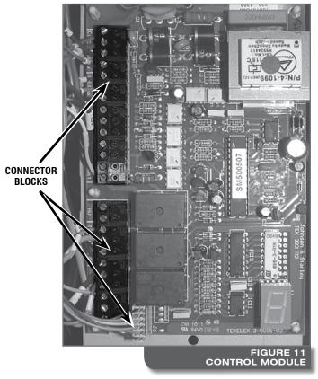
NOTE: To disconnect the module, LIFT the connector blocks off the circuit board. DO NOT remove the wires from the connector blocks!
