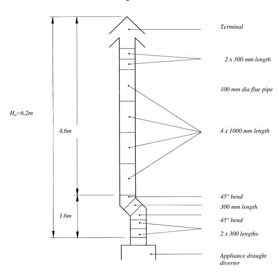
Fig. 2 Worked example of equivalent flue height
