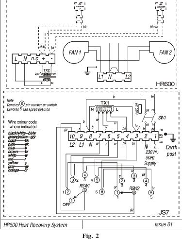
HR600 INSTALLATION WIRING DIAGRAM
