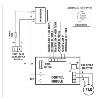
Fig. 10 HOME'N'DRY 'WALL' Wiring Diagram
