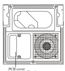
Fig. 4 Filter pad removed to expose PCB cover
