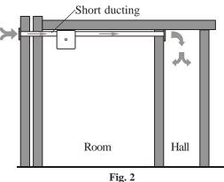
Typical installation(showing short input ducting)
