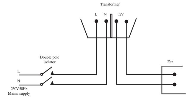
Fig. 1 A150-LV and A150P-LV Installation Wiring
