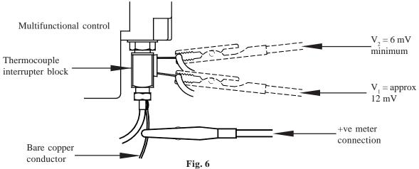
Thermocouple interrupter output check
