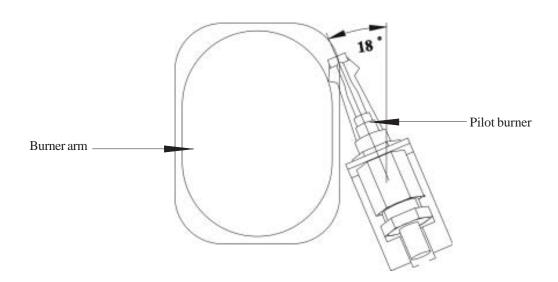
Fig. 5 Pilot assembly to Main burner relationship
