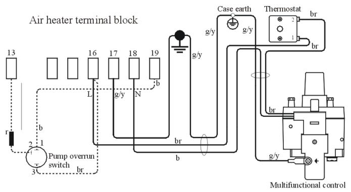
Fig. 2 SUPERJAN wiring diagram
