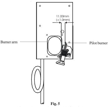
Distance between pilot assembly & main burner
