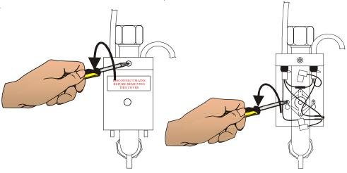
Remove the cover from the switch box assembly
