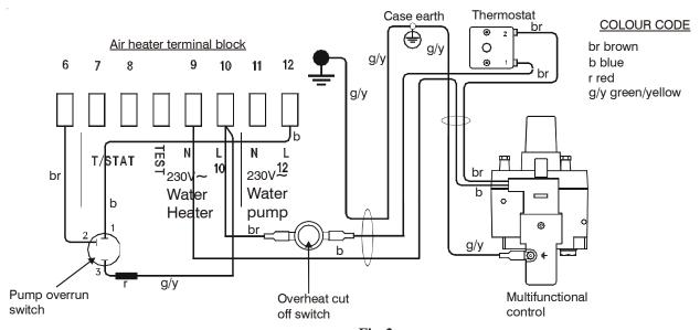
Fig. 2 SUPERJAN 6 wiring diagram
