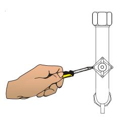
Remove the fixing bolts and completely remove the limit switch from the flow pipe.
