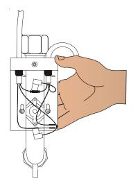
When the over-size holes are over the bolt heads, pull the switch box clear of the limit switch
