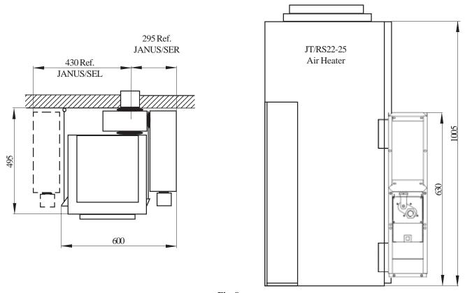
Fig. 8 JANUS SER fitted to JT/RS22-25 Air Heater dimensions (in mm)
