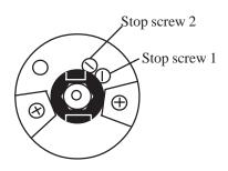
Fig. 2a Stop screw positions
