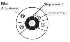
Fig. 3a Stop screw positions
