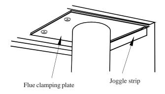
Fig. 2 ELJAN 4/SE Flue Clamping.
