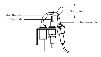
Fig. 5 Pilot burner and flame profile
