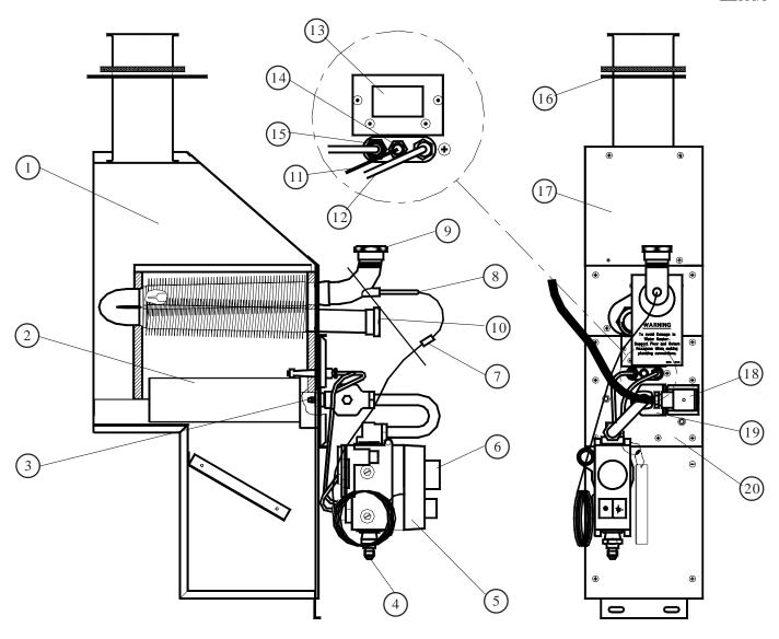
1 Circulator body 11 Electrode lead 2 Main burner assembly 12 Thermocouple 3 Main injector 13 Viewing port Gas inlet connection Igniter electrode 4 14 5 Multifunctional control 15 Pilot burner 6 Temperature control 16 Flue clamping plate Cover plate 7 Thermostat retaining plug 17 8 Thermostat phial 18 Solenoid valve coil 9 Water Flow connection 19 Solenoid valve body 10 Water Return connection 20 Burner mounting plate
