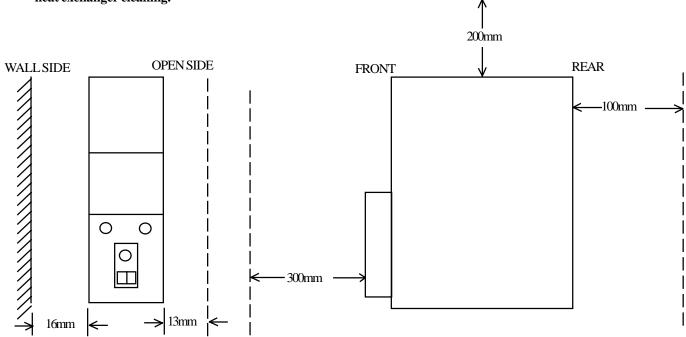
Fig. 1 Minimum clearances for ELJAN F
