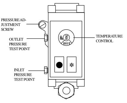
Fig. 5 Multifunctional Control Component Identification
