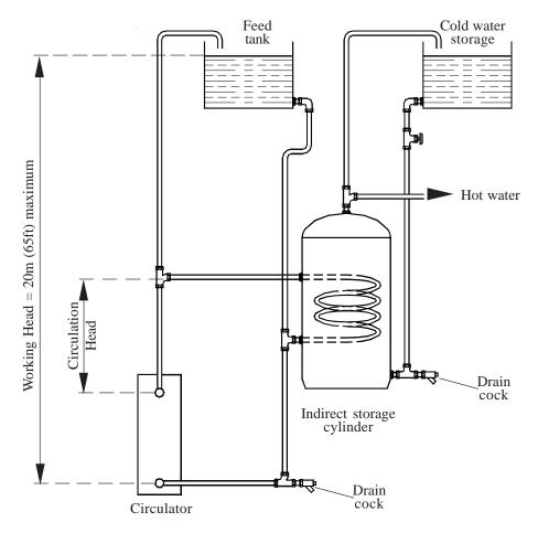
Fig. 1a. Typical ELJAN 6/HIJAN 6 Indirect System application.
