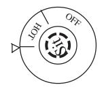
Fig. 3b Minimum Setting 60°C
