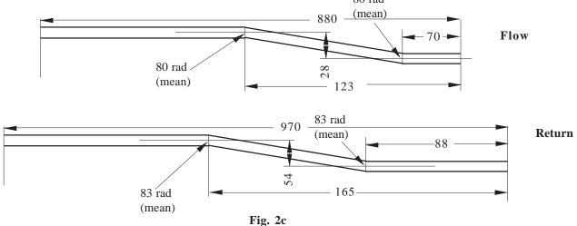
HI-SPEC M31 Top Exit Flow and Return Connection Pipes (Dimensions in mm)
