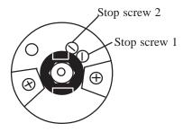
Fig. 3a Stop screw positions
