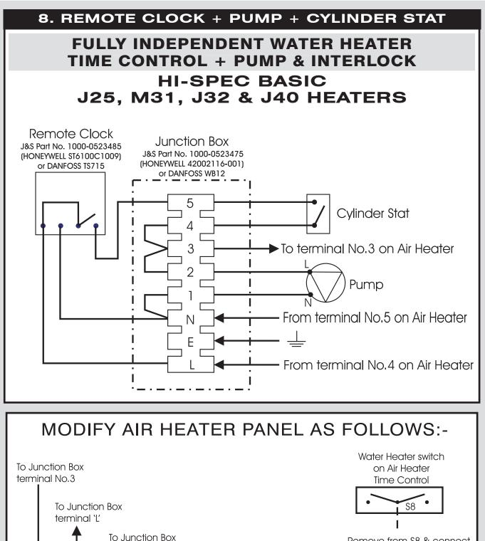
Remove from S8 & connect to terminal No.3
