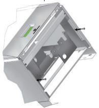
2. Place the lower cover into approximate position on top of the work surface.
