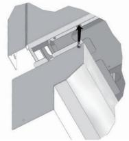
7. Using a 2.9mm drill, drill through the holes on the upper cover through the lower cover and screw into position, using self-taping screws provided in the kit
