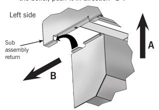
The flange on the right hand side of the upper cover mounts directly to the sub assembly but you MUST ensure that the return on the right hand side of the assembly is allowed to protrude through the slot in
