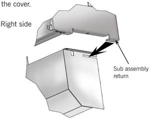
6. Once in place, secure the upper cover and both side panels with the longer screws provided in the kit.
