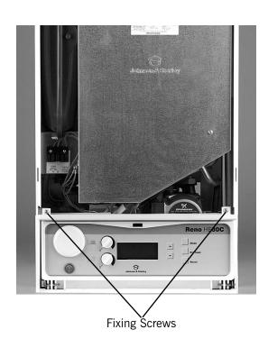
5. Remove the two fixing screws from the left hand control panel back plate, lift up the left hand end of the panel and slide the location lugs out of the slots.
