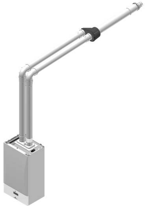
Fig.3-14 Offset Twin to Horizontal Concentric Terminal
