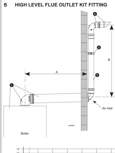
Refer to the boiler installation and servicing instructions for fitting of the boiler and its flue system.
